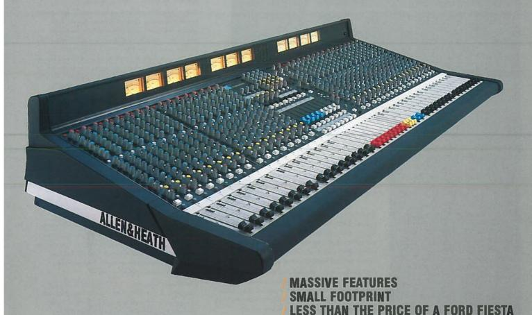
Dual Functionality / GRP/Aux mode switches reverse the group fader and aux rotary master sections to allow you to choose any combination of up to 8 Aux sends and up to 4 subgroups on fader masters with inserts and full metering. A Centre Mode switch converts the 100mm C fader to an engineer's listen wedge control with insert
